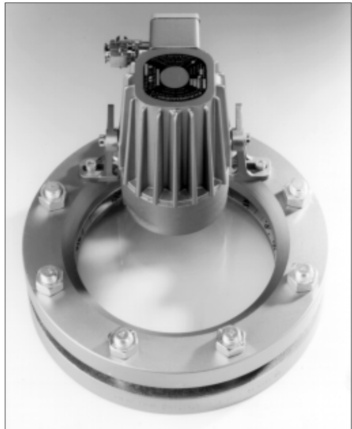
Lumiglas USL 07-Ex installed by a hinged bracket on the cover flange of a circular fitting DIN 28120, forming a combined sight/light port.
